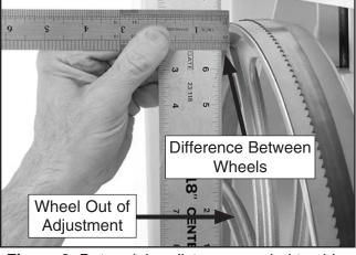
Figure 2. Determining distance needed to shim upper wheel.
